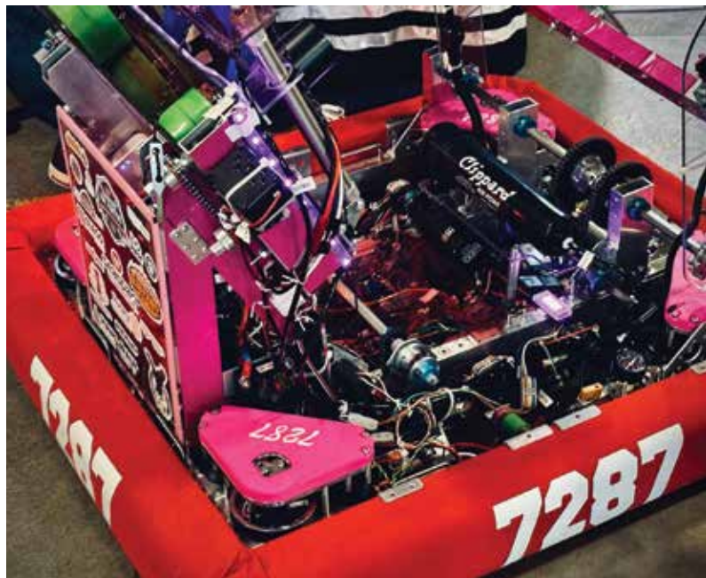
Below: Bar-B, the team’s FRC 2024 robot with signature 3D-printed pink pieces. Photos provided by author.
